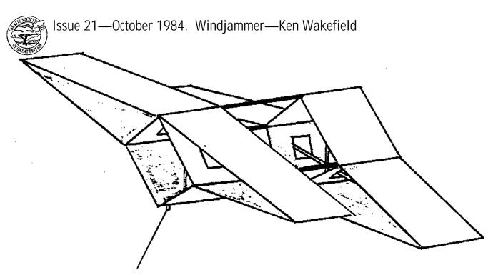
This kite is the third in a series aimed at something very large for lifting a camera rig. The lifting sails are not in line, the rear sail is lower than the front make a far more efficient set-up. The moment arm (distance between front and rear sails) is short allowing the whole kite to soar at an acute angle. Don't worry if the tips of the kite 'flex' in high winds, they are supposed to.
